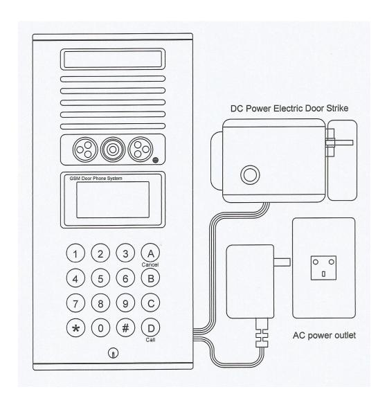
**WARNING:** Only use the original power adapter supplied. Using any other adapter might damage the door unit and cause a risk of electric shock.
