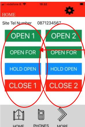
Once the Phone number is entered this first screen can be used for immediate control of the two Outputs.
